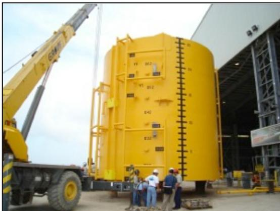
**Fig. 2.9: Buoyancy Module 2 years after installation**
