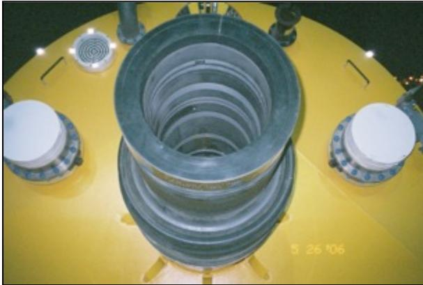
**Fig. 2.12: Suction Pile Was Used to Anchor Well Head**
