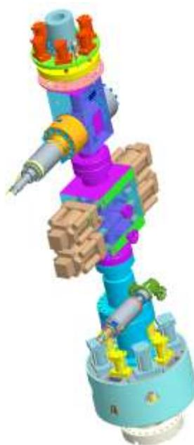
Figure 6: SSD Connected to the Wellhead
