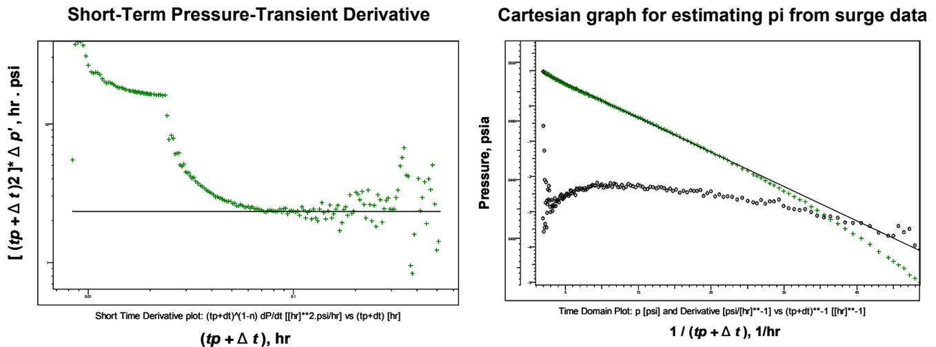
**Fig. 3 — Two plots used to determine graphically the reservoir pressure**
