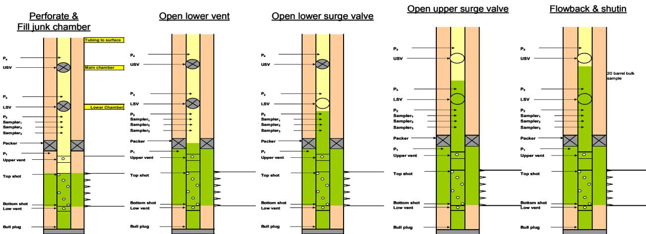
Fig. 2 - String used to start with short-term pressure-transient test and follow with a DST if necessary
