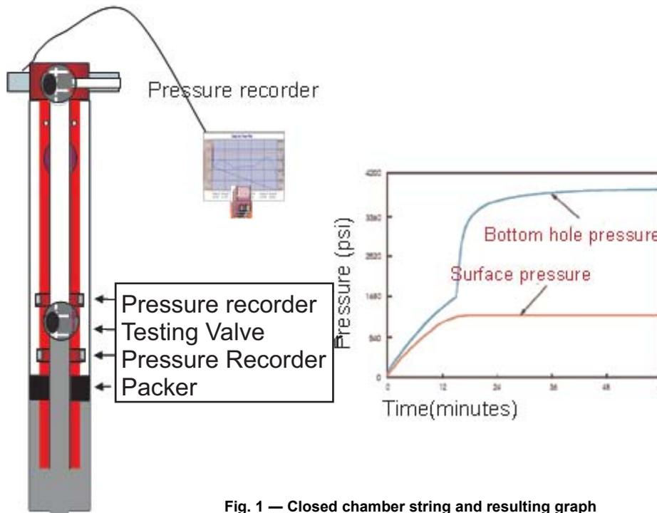
Fig. 1 — Closed chamber string and resulting graph
