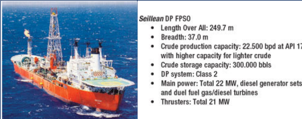
Fig. 3. The Seillean , a DP Class-2 redundant FPSO equipped for test and early production operations in up to 2,000-m water depth.
