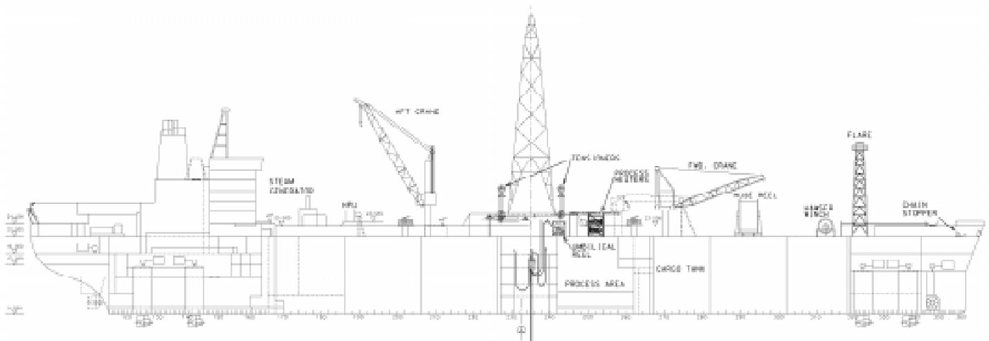
Figure 3 – FPSO Seillean – Sectional Elevation
